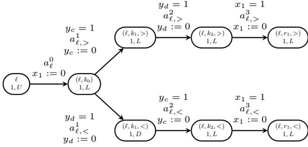
**Figure 4. Module taking into account the order between the values of  $c$  and  $d$  when incrementing  $c$ .**
